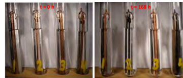
175°C for 1 week, Al, Cu, steel coupons, ASHRAE 97
